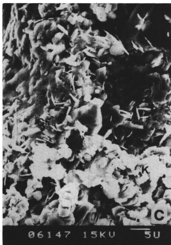
Fig. 4 - (a) Quartz overgrowth (QO) overlying Chlorit rim, scale bar 50 \mu\text{m} ; (b) Kaolinit (K) filling secondary porosity, note the vermicular form of the crystals; (c) Kaolinit as attacked pseudo-hexagonal plates and Chlorit (Ch) rim; (d) Chlorit rim in secondary pore space (see arrow).
