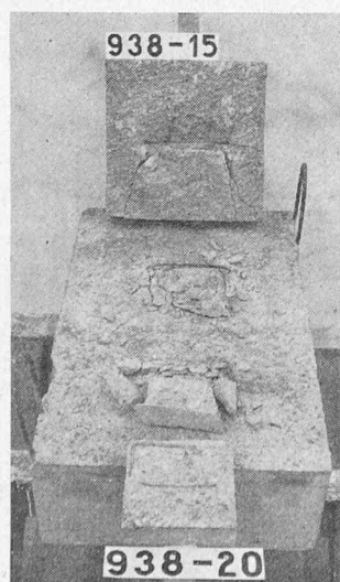
Fig. 10. Types of anchor rupture of stirrups cast into a thin concrete topping. Note the difference in type of rupture for smaller ( 15 \times 15 \text{ cm}^2 ) and larger ( 30 \times 30 \text{ cm}^2 ) surfaces. When size was (61.5 \times 61.5 \text{ cm}^2) the rupture was a pure tension cone around the stirrup
