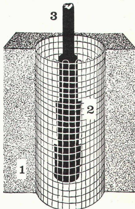
1 = Schnitt Beton 2 = Beton-Drahtkern
