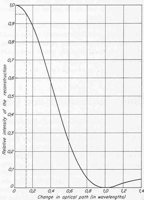
Figure 5. Effect of change in optical path during a holographic exposure (a linear change is assumed)
