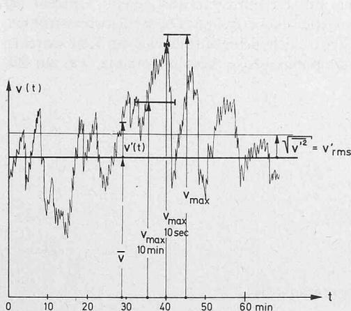
$$\bar{v} = \frac{1}{T} \int_0^T v(t) dt \quad \bar{v}' = 0$$
