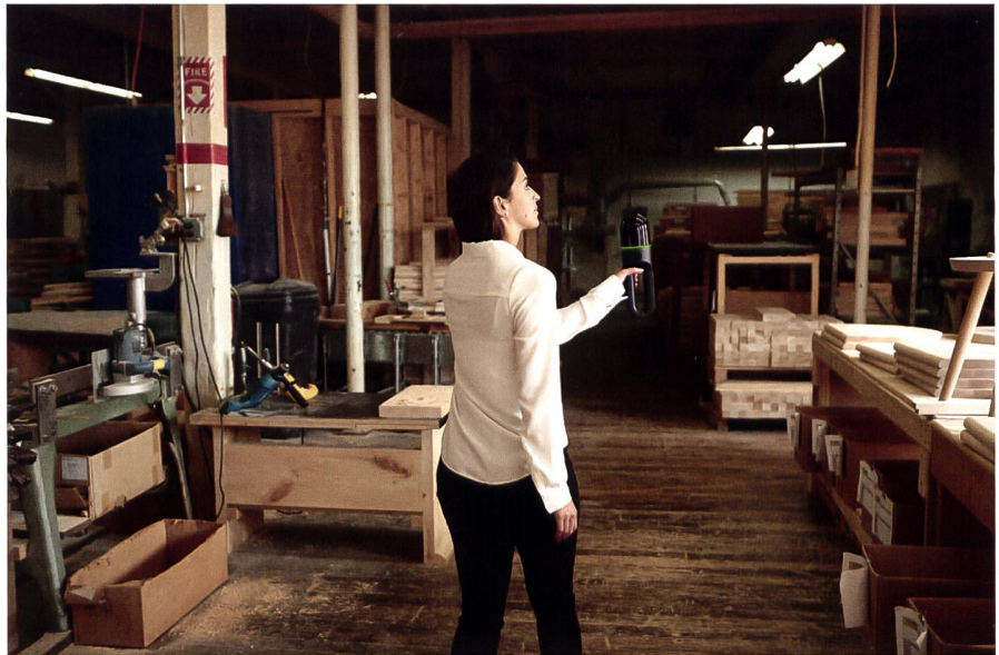
Fig. 17: The BLK2GO hand-held laser-imaging scanner digitises space in 3D while you move.
