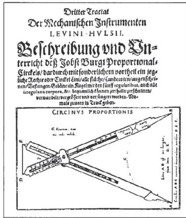
Fig. 3 Bürgi's "Proportional Circle", a precision compass device invented and built by Jost Bürgi, first mentioned by Levin Hulsius in 1603 (published in 1607). It serves to reduce the scale of an object by a constant factor (from [19], p. 130).
