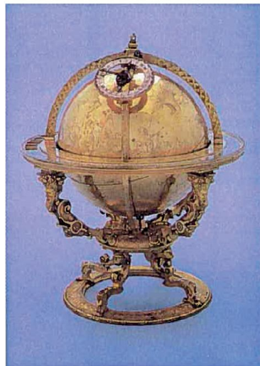
Fig. 2 The little "Himmelsglobus", completed by Bürgi in 1594, to be seen in the Swiss National Museum in Zürich, see [15], [19]. It is an extraordinary piece of early astronomy and precision craftsmanship, 142 mm in diameter and 255 mm of total height, accurately displaying the motion of the celestial sphere, the sun, and giving the time.
