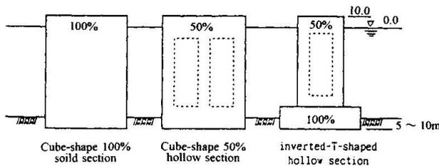
Fig. 4 Laying-down caisson used for the trial calculation
