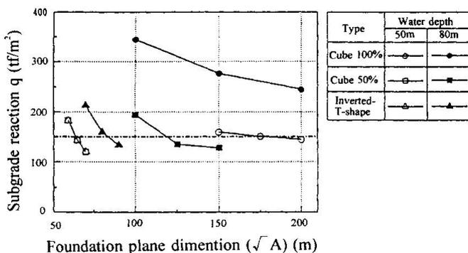
Fig. 5 Dimensions and subgrade reaction of a foundation
