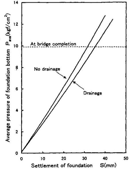
Fig. 8 Main tower foundation settlement forecast analysis
