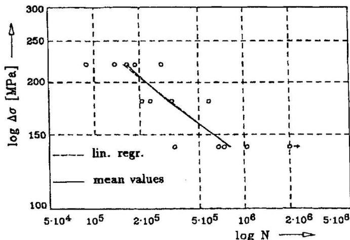
Fig. 5: Fatigue behaviour of the first test series
