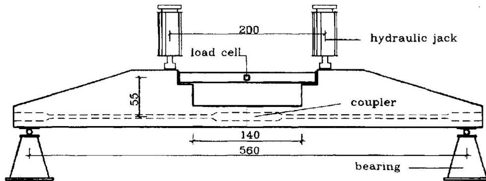
Fig. 4: Test beams for second test series
