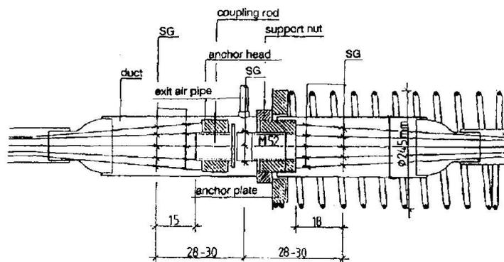
Fig. 3: Coupler B/KI, posttensioning system BBRV-SUSPA II
