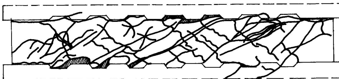
Fig.7 Cracking at collapse
