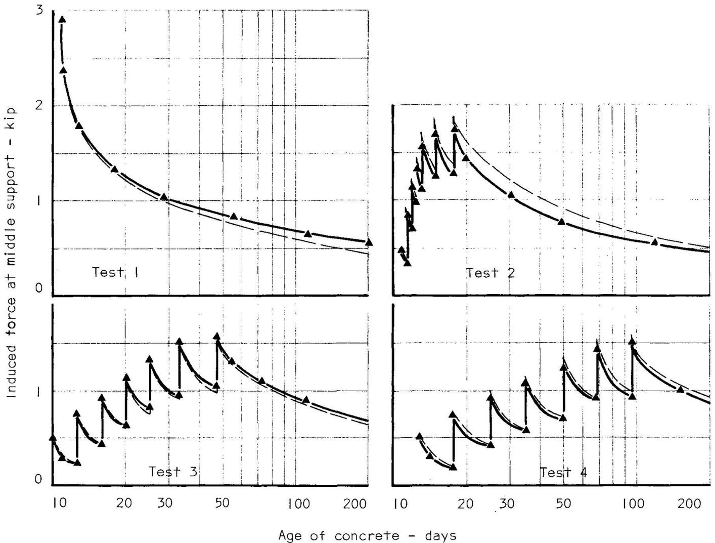
Fig. 5 Time-force relation for test beams
