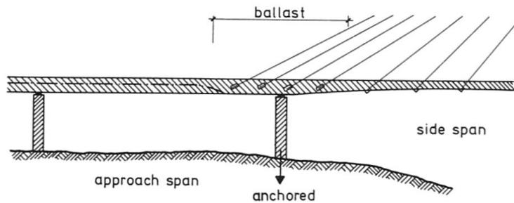
Fig. 18 Continuity to the approach bridge allows lengthwise distribution of the back stay cables
