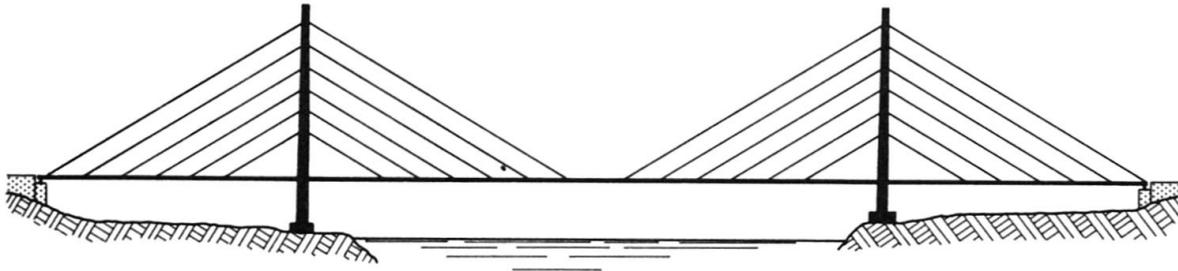
Fig. 5 Harp-shaped configuration of stay cables
