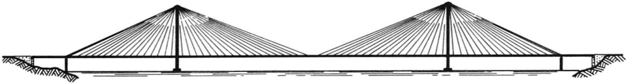
Fig. 4 Fan-shaped configuration of stay cables
