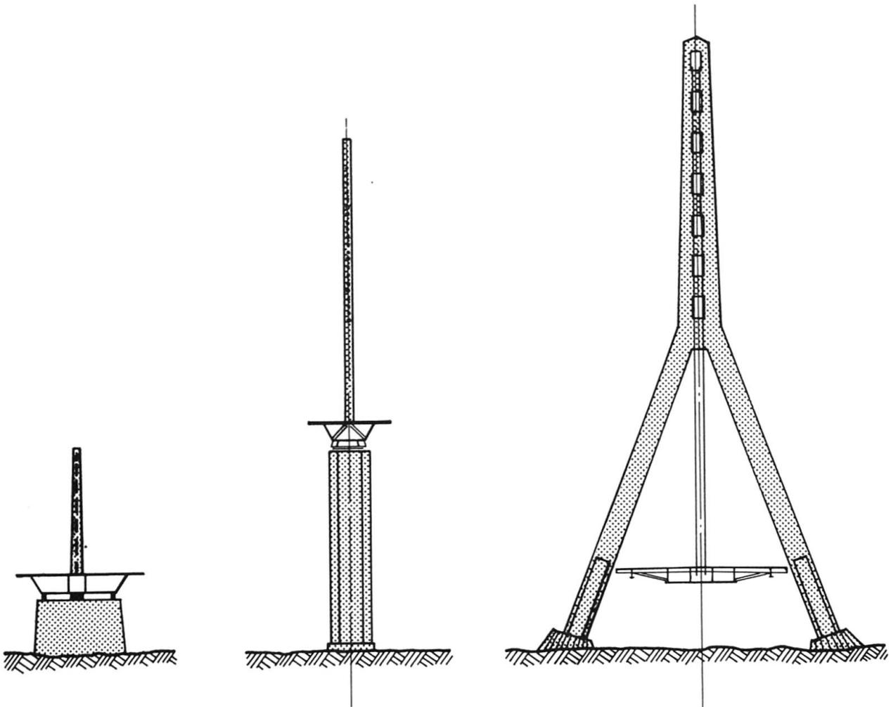
Fig. 16 One cable plane - tower shapes
