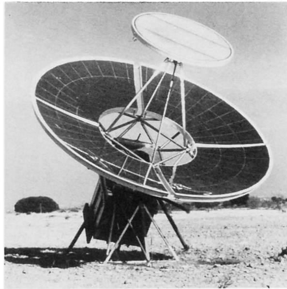
Fig. 5 A solar furnace for brick burning
