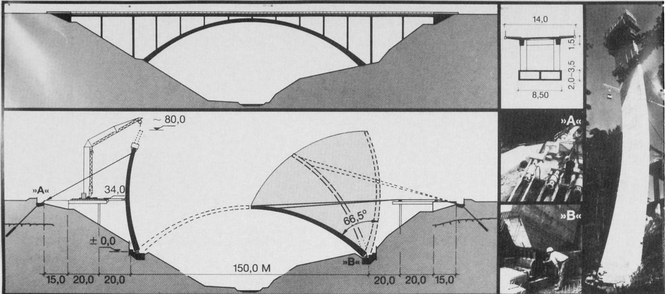
**CONCRETING:** accuracy  $\pm 3$  cm, climbing formwork, 27 sections 81,5 m within 3 months
