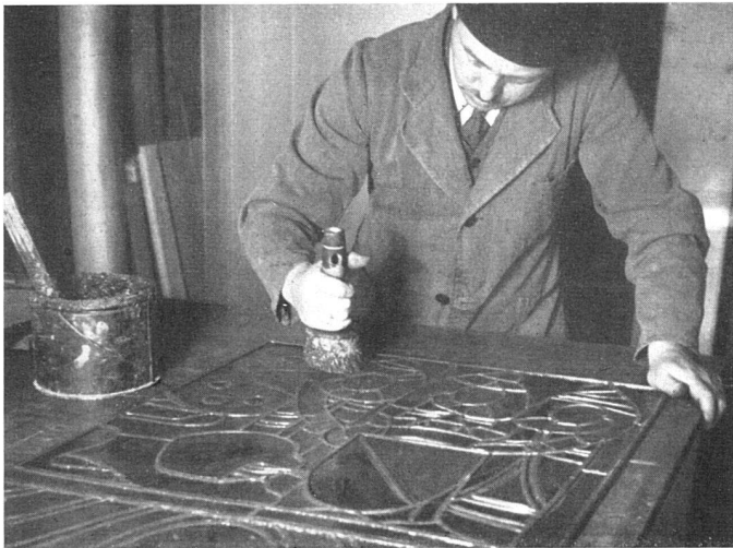
12 Das Kitten | Masticage du vitrail | Puttying of window
