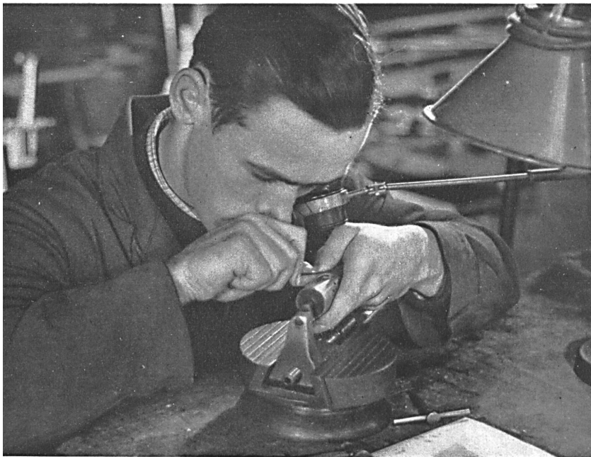
Hand-engraving in relief on a steel roller which, in its turn, will be used to sink the design into a copper cylinder for rotary printing.
