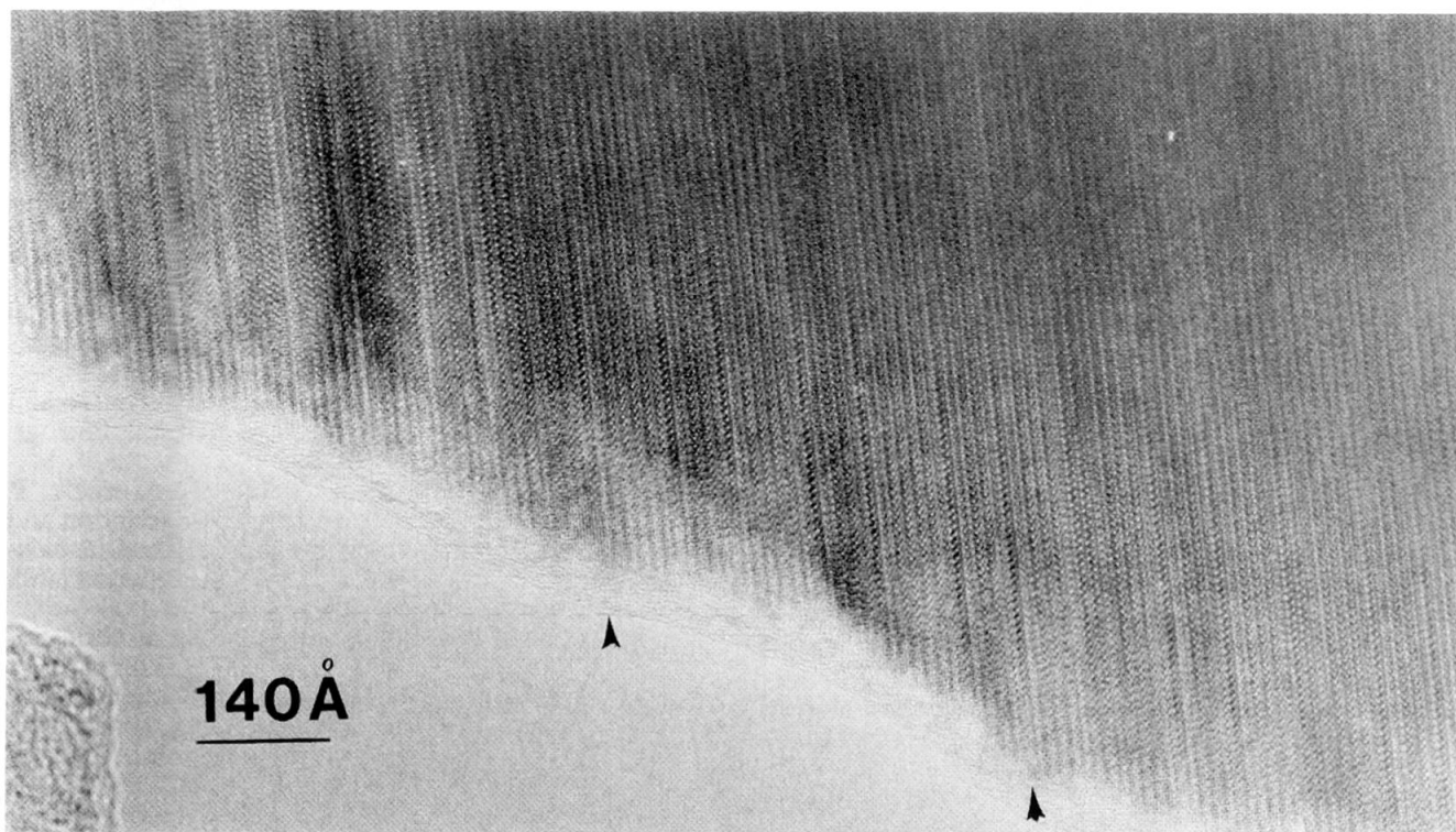
Fig. 15 Electron micrograph showing polysomatic disorder in a sartorite group mineral. The central section of the image (between the black arrows) contains 3 repeats of the 138 Å phase. The modules sequence in the rest of the image is disordered.
