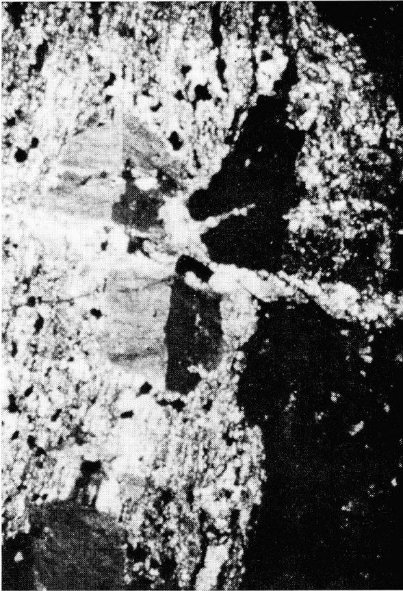
Photograph 1 (width: 3.3 mm). Dacitic rock component, sheared during Alpine deformation, with primary uranium minerals (lower part of photograph).
