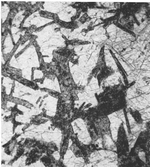
Photo Nr. 4. Coarse ophitic diabase. Main rock type of Gorgona island. Idiomorphic plagioclase laths and augites. Enlarg. approx. 90 ×
