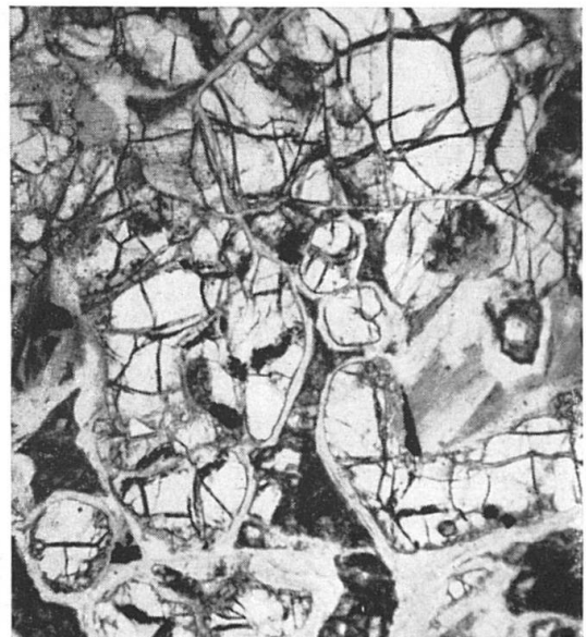
Photo Nr. 5. Peridotite from Gorgonilla Island. The olivines are partly altered into serpentine. Enlarg. approx. 90 ×.
