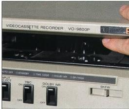
The playback equipment should be clean and in good working order. Take a look in the cassette slot – is it empty and dust-free? You can remove loose dust using compressed air (e. g. from an aerosol) and a powerful vacuum cleaner. Never touch the **head drum** or the **tape guides**. Always ask a specialist or a professional technician to remove stubborn dirt, and also to service the device at regular intervals.
