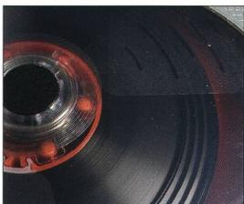
Does the **tape pack** show stepping or unevenness? If so, wind and rewind the tape from one end to the other. If the tape sticks or **squeals** while it is being wound or rewound, stop the winding process immediately. If you suspect the tape is afflicted by *>Sticky Tape Syndrome*, give it to a video conservator without attempting to view it.
