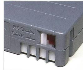
**Video8**, **Hi8**, Digital8: there is a sliding tab on the side of the cassette, which should be moved to the closed position.
