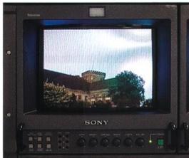
Protect your CRT monitor from magnetic fields, too. For example, do not position it in the immediate vicinity of headphones, active speakers or other hardware that generates magnetic fields, or colour shifts may occur on the display.
