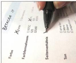
Prior to viewing the tape, compile all relevant technical information. Read all the labels on the cassette shell and case and study the attached **dub sheet** – if present – as well as any other reference material or documentation. Use the 'Data Sheet for Cataloguing Videotapes' as a guide and note down all available information before viewing the tape.
