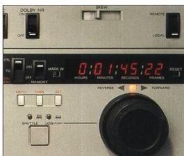
If the tape has **time code**, this will automatically appear on the player's display while the tape is playing (set the switch to TC). If no time code has been recorded on the tape, you should manually set the tape counter to 00:00:00 either at the start of the tape or at a desirable point along the tape (set the switch to CTL and press the reset button).
