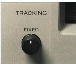
If the player is fitted with a **tracking control**, set it to the neutral position before viewing the video.
