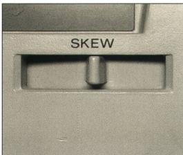
U-matic players have a control for adjusting the **tape tension**, known as a **skew control**. Before viewing the tape, make sure this control is switched to the neutral position (cf. *>Skew Error*).
