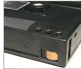
MII, DV, MiniDV, DVCAM, DVCPRO, HDV, DVCPRO HD; often also **VHS**, **S-VHS**, **VHS-C** and **S-VHS-C**: there is a sliding tab on the side of the cassette, which should be moved to the open position.
