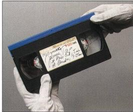
Never touch the **magnetic tape** with bare hands, because any trace of fingerprints or other contaminants may cause **dropouts**. Before inspecting a tape, it is a good idea to wash your hands or wear clean gloves. This also helps to protect the cassette shell and any labels, which are often designed or inscribed by the artists themselves.
