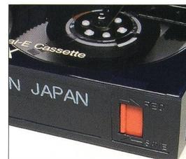
All analogue and digital cassettes in the **Betacam** family, as well as MPEG IMX, HDCAM and HDCAM SR cassettes: on the underside of the cassette is a red latch which should be pressed down.
