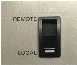
Professional videotape players from **U-matic** onwards have what is known as a remote switch, which can be used to select whether the unit is operated directly ('local' setting) or from an external control system ('remote' setting). Check that this switch is in the correct position.
