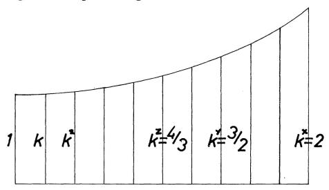
It was also desired that one string should be nearly  $\frac{3}{2}$  times and one nearly  $\frac{4}{3}$  times as long as the first string. We then have to find three integers x, y and z such that
