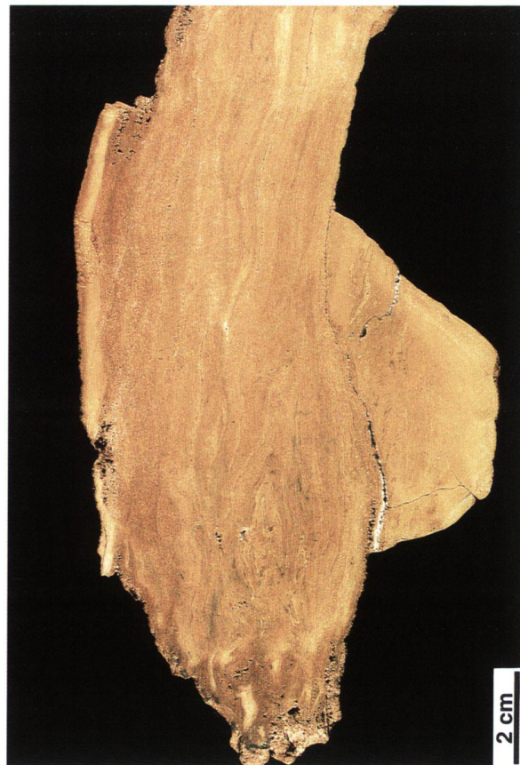
Fig. 3. Cross-section of a quartzite hand sample showing the undulously laminated structure. Laminae have thicknesses up to 1 cm.
