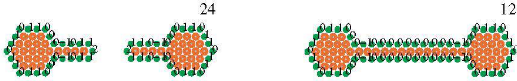
Fig. 13 Joining two regions changes the total curvature by 12. One can prove this by trimming both sides. The left-hand side trims down to a disconnected domain consisting of two discs of radius 1, the right-hand side will end up with a disc of radius 1.
