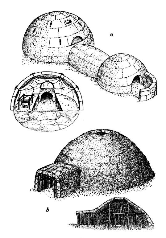
PRIMITIVE DWELLINGS, viewed as engineering structures, extract remarkably high performance from commonplace materials. Eskimo igloo (a) is built from snow blocks 18 inches thick that have insulating value equivalent to two inches of glass fibres. When lined with skins (detail drawing) the temperature of the interior can be raised to 40 degrees F without melting the dome. Summer house of Nunamiut Eskimos (b) follows igloo plan, but is made of sticks covered with slabs of turf.
