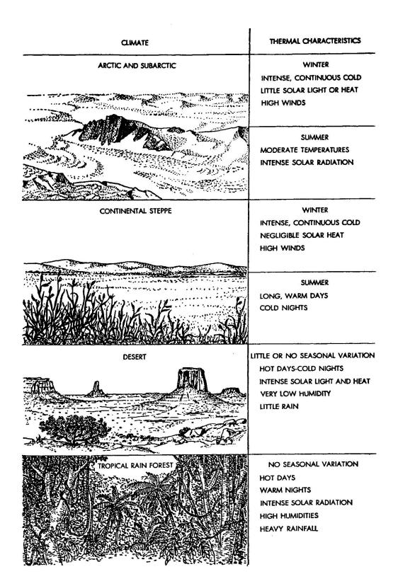
IMPACT OF CLIMATE and available building materials on the design of primitive dwellings is summarised in this chart. It describes the four climatic regions where the greatest variety of primitive architecture is still to be found. In the first three climate zones, control of temperature is the crucial architectural problem. In the fourth heavy seasonal rains add to the difficulty.
