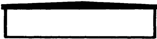
Tapered Beam Width: 28' through 80' Height: 10' through 20' Slope: 1:24
