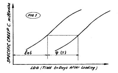
Hence knowing the specific creep curve at one temperature for T.S material one can determine the specific creep curves for that material at any other constant temperature T, by simply replacing the argument t in reference curve by t  $\not a$  (T).
