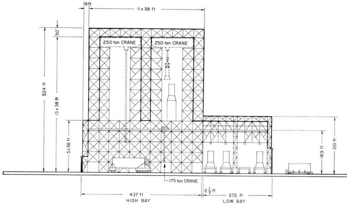
Fig. 16. North-South Section along transfer aisle of V.A.B.
