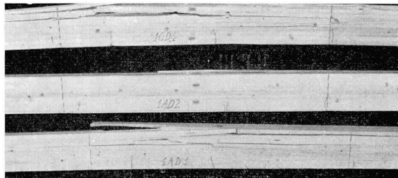
Fig. 6. Beams Loaded to Failure.
