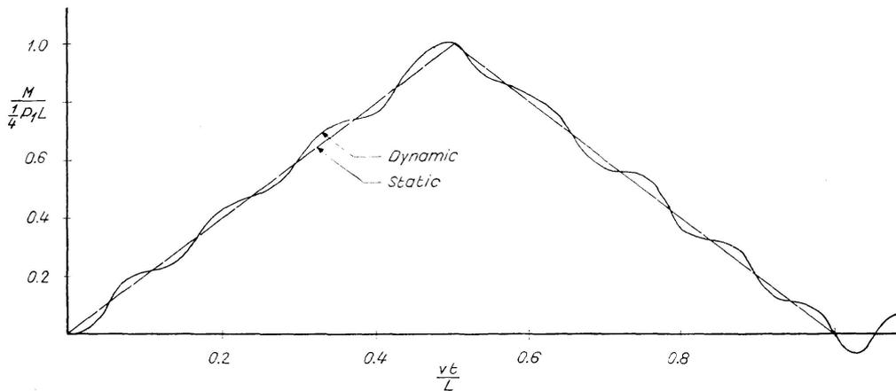
Fig. 4. Bending Moment at  $x/L = 0.5$  (plotted against time).
