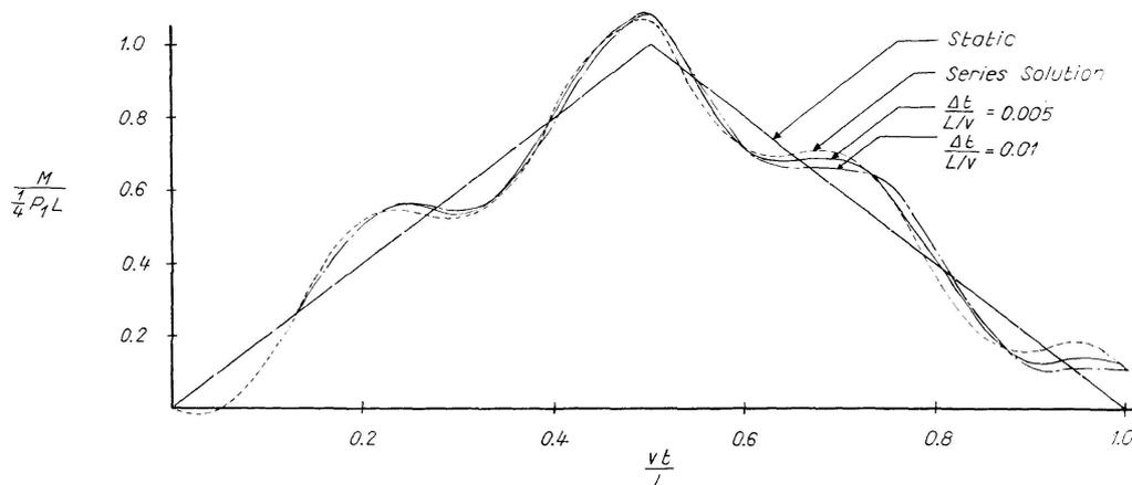
Fig. 2. Bending Moment at  $x/L = 0.5$  (plotted against time).
