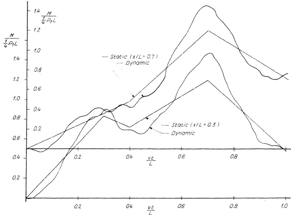
Fig. 5. Bending Moment at  $x/L=0.3$  and  $x/L=0.7$  (plotted against time).
