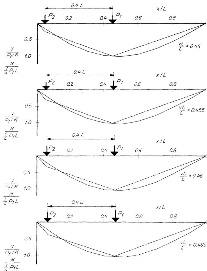
Fig. 3. Successive Instantaneous Bending Moment Diagrams --- and Deflection Curves — (obtained from the difference equations)
