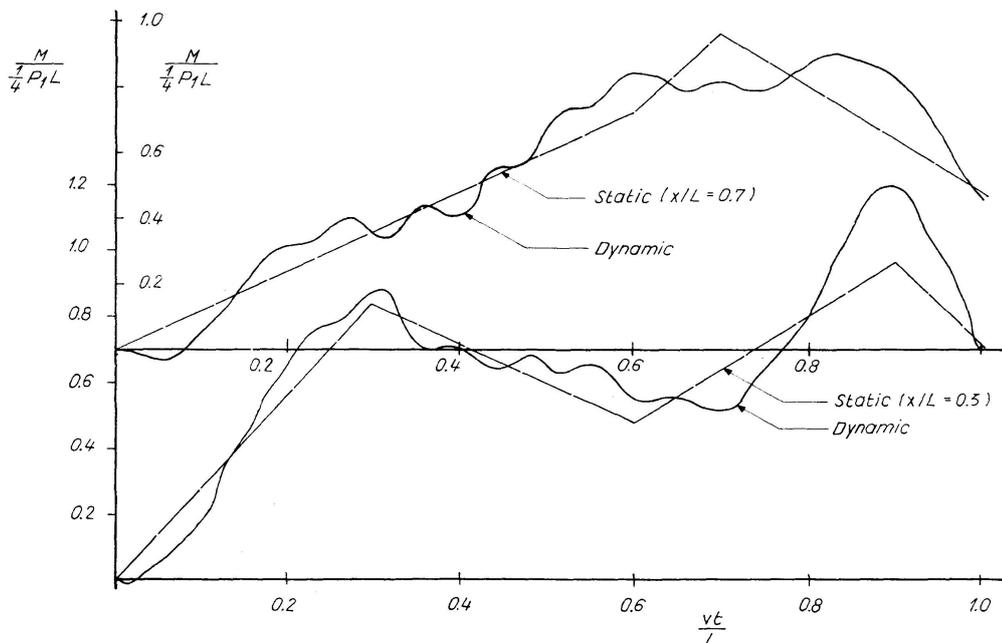
Fig. 6. Bending Moment at  $x/L=0.3$  and  $x/L=0.7$  (plotted against time).
