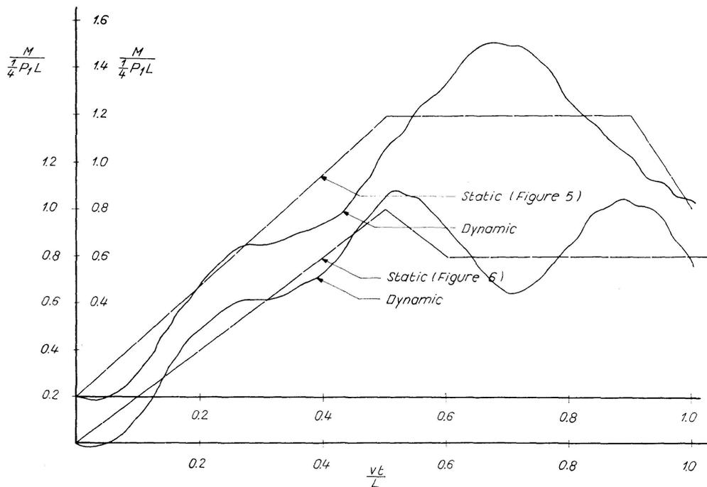
Fig. 7. Bending Moment at  $x/L = 0.5$  (plotted against time).
