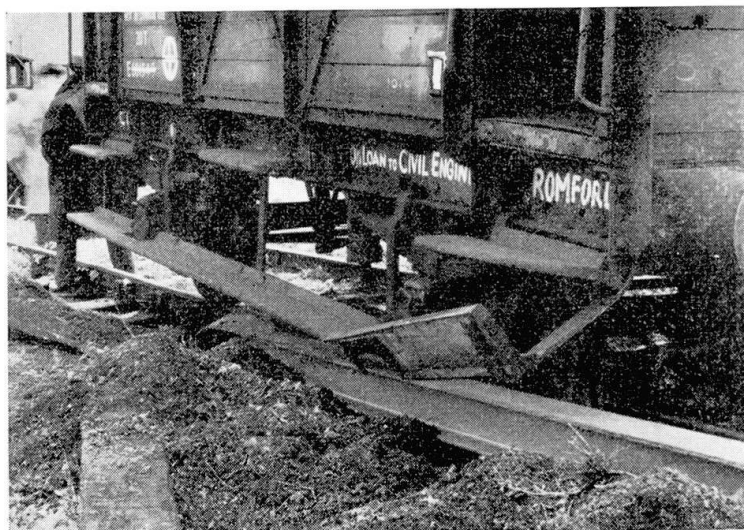
Fig. 4. Romford Impact Tests. Steel Mast After Direct Impact.
