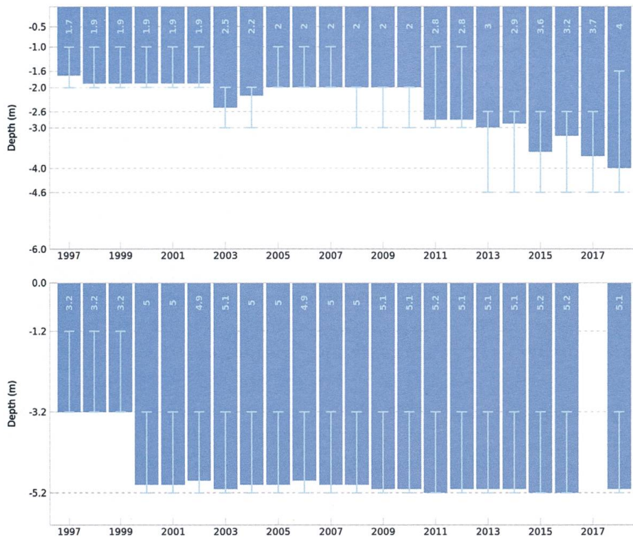
Fig. 2: Maximum annual active layer thickness (top) in an ice-poor talus slope on the Muot da Barba Peider ridge (Pontresina, Canton Grisons) between 1997 and 2018 and in the ice-rich Schafberg rock glacier nearby (bottom), between 1997 and 2018. Light blue bars indicate thermistor depths used for linear temperature interpolation (Data: SLF/PERMOS).
