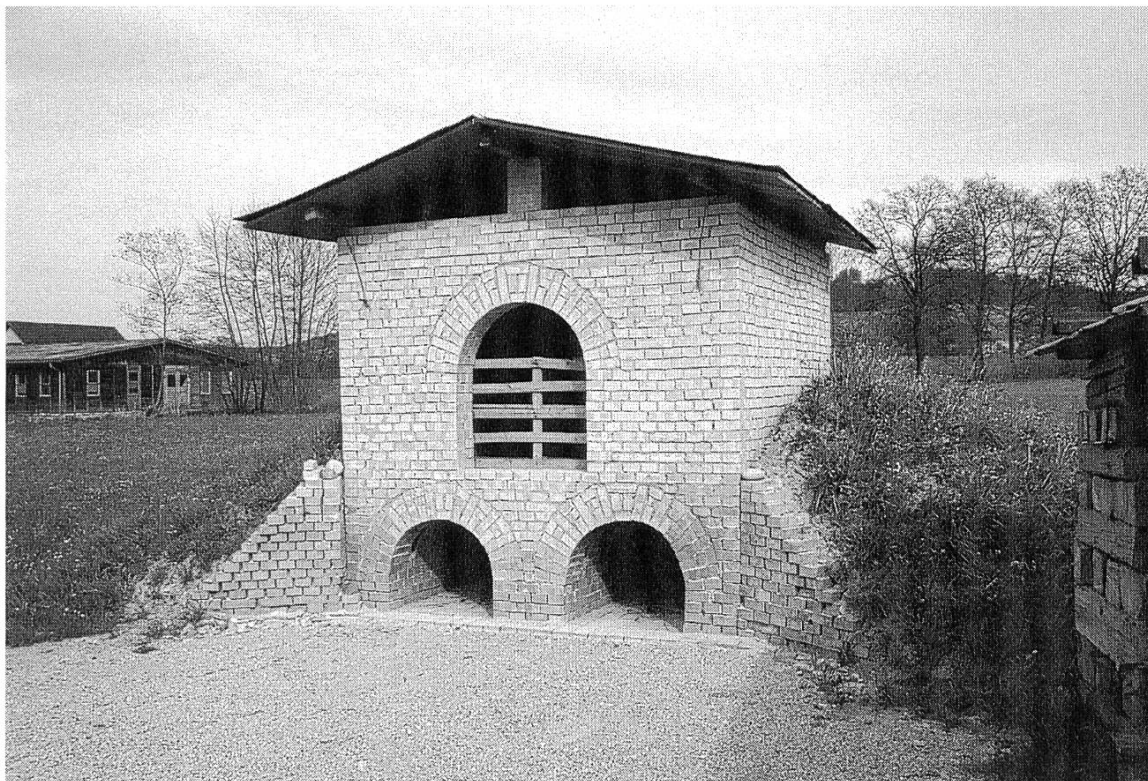
Abb. 1 Ofen des Backstein- experiments in St. Urban
