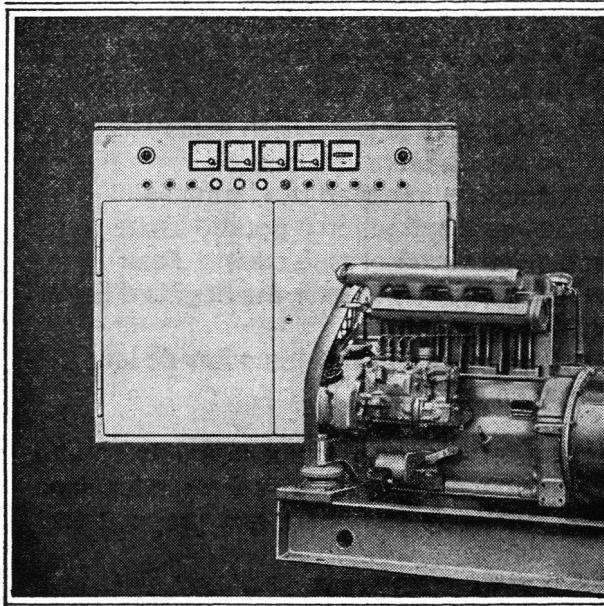
Diesel-Notstromaggregat 25 kVA, 50 Hz, 380 V
