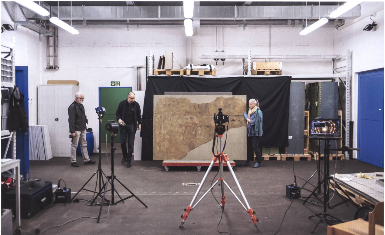
Figure 8. Setting during the photogrammetric photography in the SNM Collection Centre.
