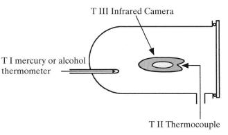
Fig. 6 Present temperature measurements during plasma treatment T I-T III:
