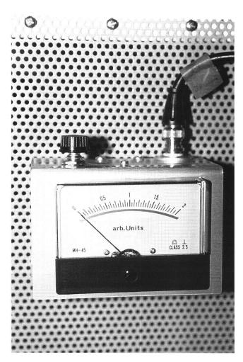
Fig. 2 Plasma current instrument.
