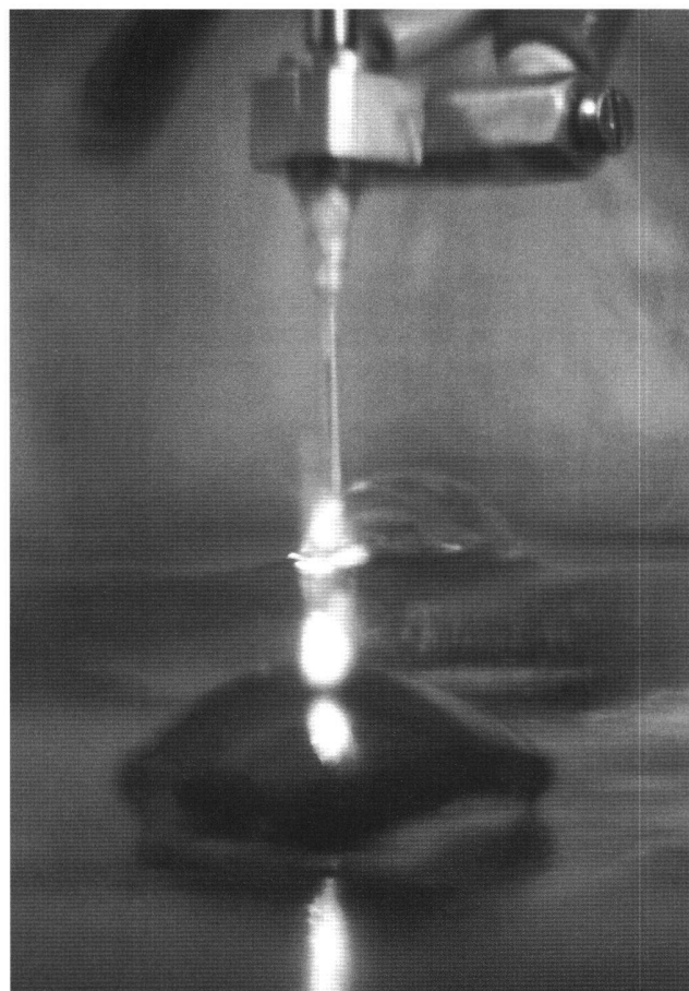
Fig. 1 Plasma pencil – RPJ in combination with 1% solution of Complexon III for applications on
