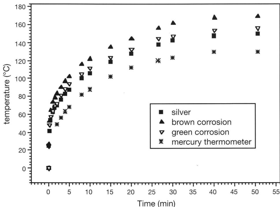
Fig. 1. Temperature measurement during plasma treatment of silver coins in hydrogen plasma ( $p = 100$  Torr,  $Q = 30$  sccm,  $P = 200$  W). Three thermocouples were sealed to the different parts of the coin.
