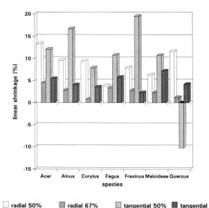
Fig. 4 Average shrinkage (%) of stabilized and non-stabilized boards in radial and tangential fibre direction (n = 2 per species, treatment, and direction).
