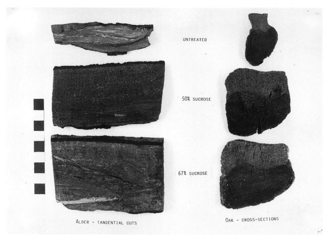
Fig. 2 Dimensions of untreated air-dried samples and samples stabilized in 50% or 67% sucrose solutions. The three comparison samples originated from the same piece of wood. Basically, the effect of sugar conservation on the stabilization of heavily degraded wood is a positive one; however, there is an obvious difference between the 50% and 67% samples.
