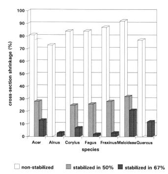
Fig. 3 Average cross-section shrinkage (%) of stabilized and nonstabilized samples at 40% rh (n = 3 per species and treatment). Due to a large number of cracks, the values of the alder and oak treated in 50% sucrose could not be calculated with satisfying accuracy; thus they were deleted.
