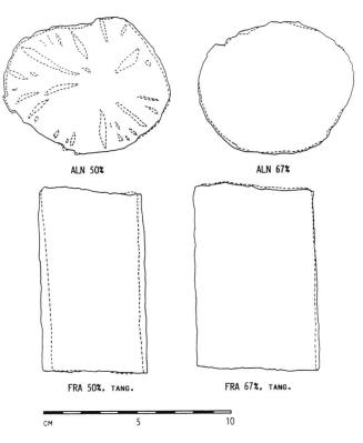
Fig. 5 Contours of samples before and after the stabilization in a 50% or 67% sucrose solution (a choice of representative samples only).
