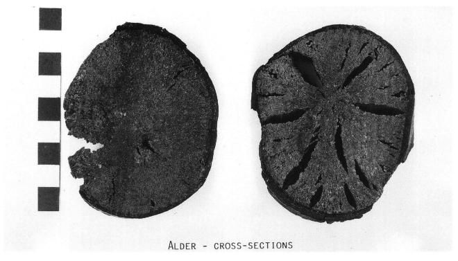
Fig. 7 The two sides of a cross-section stabilized in a 50% sucrose solution. The concave bottom side shows a number of major cracks while only a few are visible on the convex upper side.
