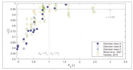
Figure 2.2: Relative discharge reduction  $\eta = C_{dH}/C_d$  at standard ogee weir profile due to LW blockage as a function of relative weir pier overhang  $P_K = p_K/H_o$  for data from this study with log diameter classes A (0.37 m), B (0.2 m), and C (0.54 m) as well as from Hartlieb (2015) and Bénet et al. (2021).
