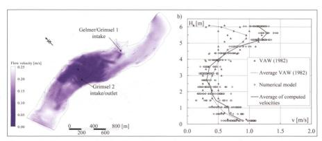
Figure 4.2: Volumetric distribution of flow velocity and computed flow velocities at the trash rack of Grimsel 2 intake/outlet structure for turbine operation (Müller et al., 2018).
