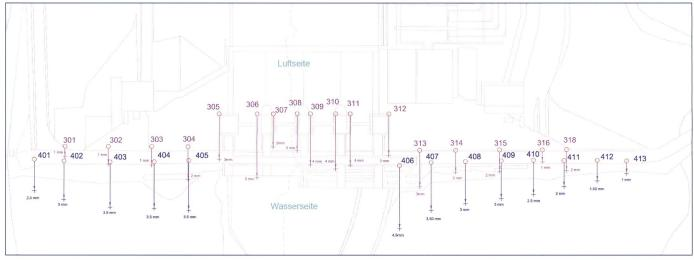
Figure 11. Ulza HPP with vertical displacement vecotrs.
