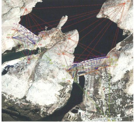
Figure 4. Geodetic Network for Vau I Dejes HPP (with Zadeje and Qyraq dams), reference points and lines of sight in red and green, object points and lines of sight in blue, levelling points and lines in purple.
