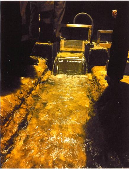
**Figure 2. Automated rectangular weir measuring seepage flow inside Komani dam.**
