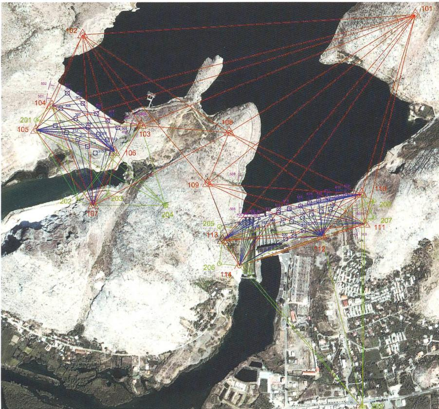
**Figure 4. Geodetic Network for Vau I Dejes HPP (with Zadeje and Qyraq dams), reference points and lines of sight in red and green, object points and lines of sight in blue, levelling points and lines in purple.**
