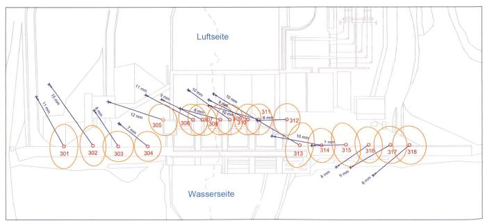
Figure 10. Ulza HPP with horizontal displacement vectors and confidence ellipses 95%.
