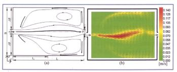
Figure 6. (a) Time averaged flow pattern and velocity magnitude (m/s) with sediment entrainment flow obtained by LSPIV measurements after 4,5 hours, (b) Plan view of the reference experimental setup (L=6 m, B = 4 m). Discharge Q = 7.0 l/s, water depth  $h = 0.2 \, \text{m}$ , and suspended sediment concentration  $C = 3.0 \, \text{g/l}$ .
