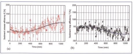
Figure 9. Evolution of sediments release E (left) and trap efficiency T (right) for long run duration (18 hr).
