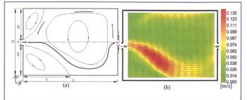
Figure 5. (a) Time averaged flow pattern and velocity magnitude (m/s) for clear water obtained by LSPIV measurements, (b) Plan view of the reference experimental setup (L=6 m, B=4 m) and definition of the geometrical parameter of the first recirculation cell in the basin (Lr). Discharge Q = 7.0 I/s, and water depth h = 0.2 m.
