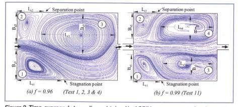
Figure 2. Time-averaged streamlines obtained by LSPIV measurements for clear water flow for two different basin geometries with shapes  $f = (A/P^2)*ER$  of 0,96 (left) and 0,99 (right). The geometrical parameters of the recirculation cells in the basin are  $L_{ri}$ ,  $B_{ri}$  for gyres (1, 2, 3 and 4).
