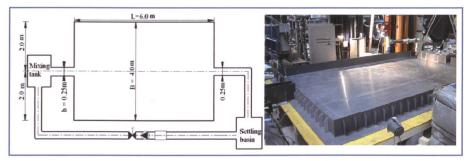
Figure 1. (a) Plan view of the reference experimental setup (L=6 m, B=4 m); (b) photograph, looking downstream.
