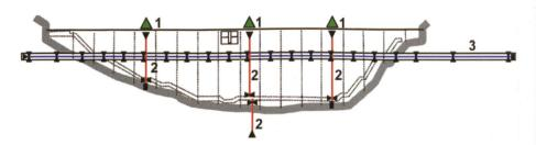
Figure 7. Device for measuring deformation of a gravity dam. 1. Geodetic pillars, 2. pendulums, 3. wire alignment.
