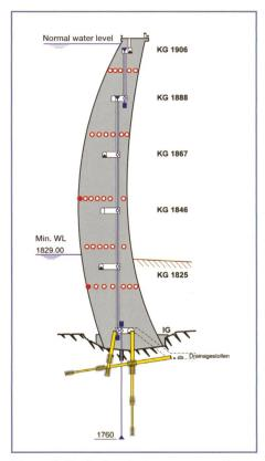
Figure 3. Typical arch dam cross section.
