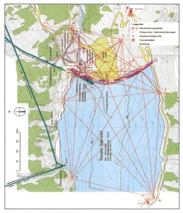
Figure 4. Geodetic network.
