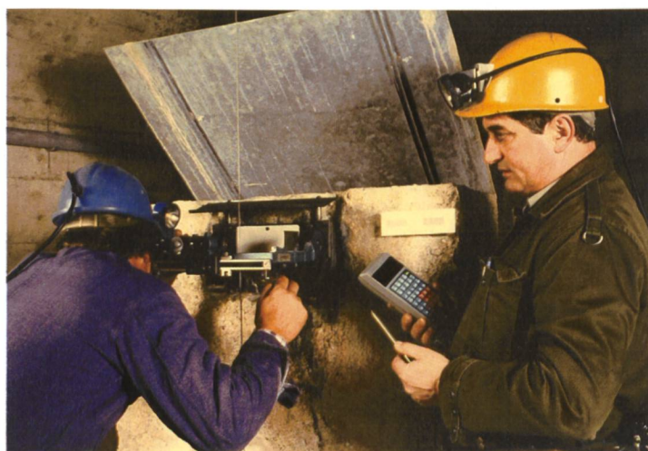
Figure 8. Measurement of pendulum deformation in a dam gallery. (Source: Emossan SA).
