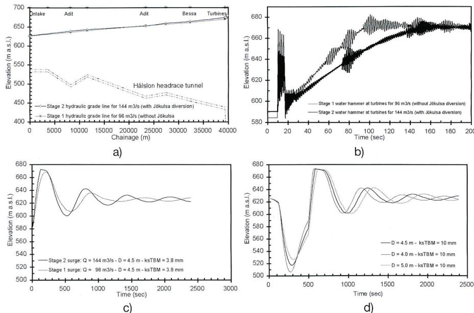
**Fig. 3. Results of the transient calculations: a) Hydraulic grade lines for stage 1 (96 m<sup>3</sup>/s) and stage 2 (144 m<sup>3</sup>/s) closing procedures; b) Corresponding water hammer at turbines; c) Surge tunnel oscillations for stage 1 and stage 2 closing procedures and a tunnel diameter of D = 4.5 m; d) Surge tunnel oscillations for stage 2 opening-closing procedure and different surge tunnel diameters.**
