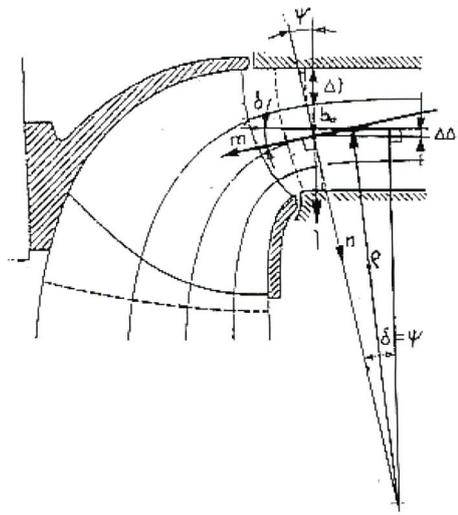
**Fig. 1. Guide vane outlet-flow towards the runner inlet for calculation of the blade-inlet angles for the different stream surfaces. (Note: n-direction is normal to the meridian flow direction with positive value towards the centre of the curvature radius  $\rho$ .)**
