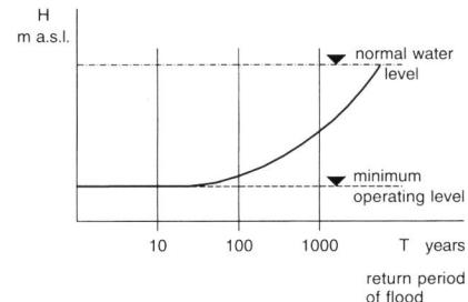
Figure 19. Filling of an empty reservoir in case of flood (with bottom outlets fully open).
