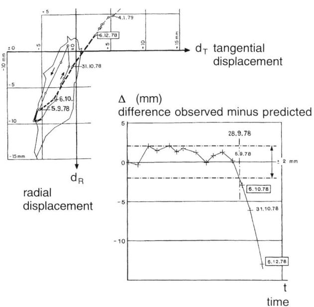
Figure 10. Abnormal ground settlement in the area of the reservoir of Zeuzier: displacement of the fixing point of the middle plumb line.
