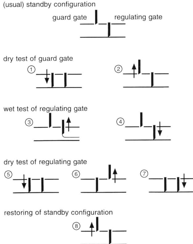
Figure 8. Operating test of a double gate.
