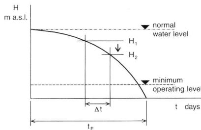
Figure 18. Time required to partially or totally draw down a reservoir (with bottom outlets fully open).
