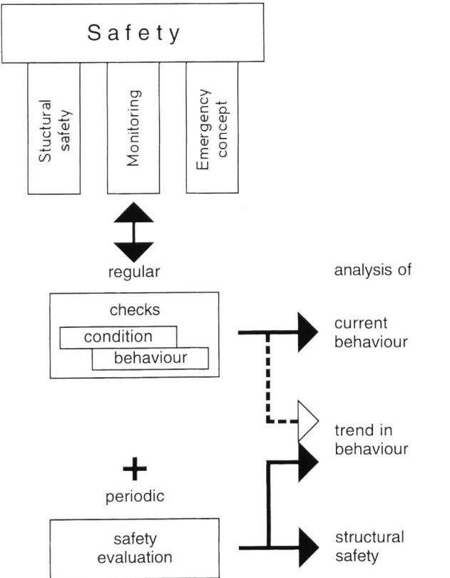
Figure 6. Elements of surveillance and objectives.
