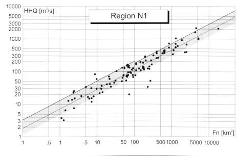
$Q_{\text{max}} = 13,18 \cdot Fn^{0.6} \text{ (Fn} \le 100 \text{ km}^2\text{)}$  $Q_{\text{max}} = 12.02 \cdot Fn^{0.6} (Fn > 100 \text{ km}^2)$  $Q_{\text{max}} = 56,23 \cdot MQ^{0.62} \, (MQ \le 3 \, \text{m}^3/\text{s})$
