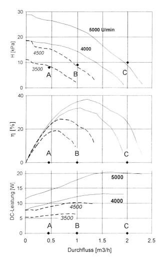
\_\_\_\_ Motor 10 W/Laufrad B28Z ---- Motor 5 W/Laufrad R25Z
