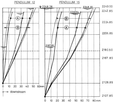
Figure 3.4. Upstream-downstream displacements of a point on the pendulum as a function of the reservoir level
