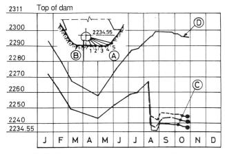
Figure 3.6. Uplift pressures observed at the toe of Naret 1 Dam as a function of time:
