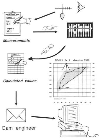
Figure 6.1. From the eye of the dam warden to the analysis by the engineer: the lengthy measuring chain.
