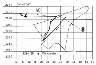
Figure 3.7. Average coefficient of uplift pressure in a transverse section of Naret 1 Dam
