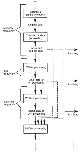
Figure 5.1. Principle of the measurement chain.
