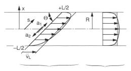
$$\overline{v}_{L} \ = \ \frac{1}{L \, cos \theta} \int_{s = L/2}^{s = t/2} v(s) \, cos \theta \, ds = \ \frac{1}{2R} \int_{x = R}^{x = t} v(x) \, dx$$
